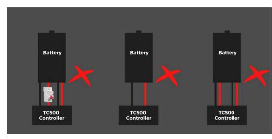
Use only tools and screws that came with the controller. Using the tools and screws that were not included in the parcel, not following these instructions, or not using the circuit breaker or a fuse, can cause serious damage to you and your bike, and voids your 2-year warranty.
