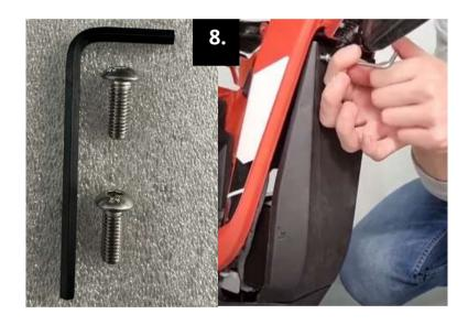
STEP 8: Use the longer M6 screws and a larger hex key to fasten the shield to the frame.
