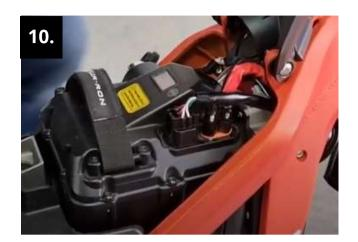
STEP 10: Connect the battery to the battery power connector and the 6-pin connector.
