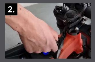
Now you can start removing the stock SurRon controller and the battery from the frame, and lower the skid plate that covers the wiring.
